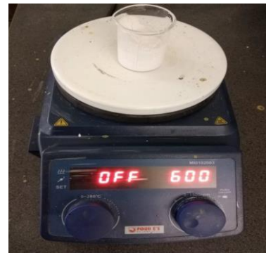
Fig. 2.4 Preparation of slurry by magnetic stirrer
