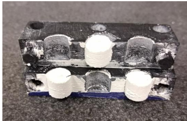
Fig. 2.5 The prepared ceramic green bodies after de-moulding
