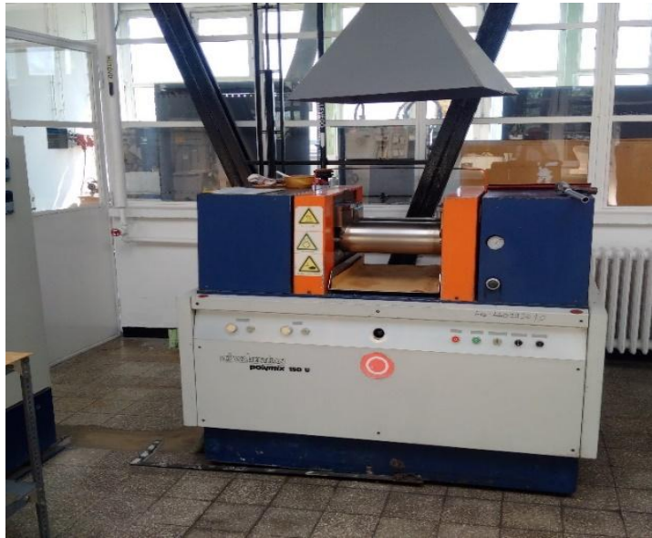
Figure 8. Schwabenthan UL 150 electrically heated two-roll mill used for blend preparation.
