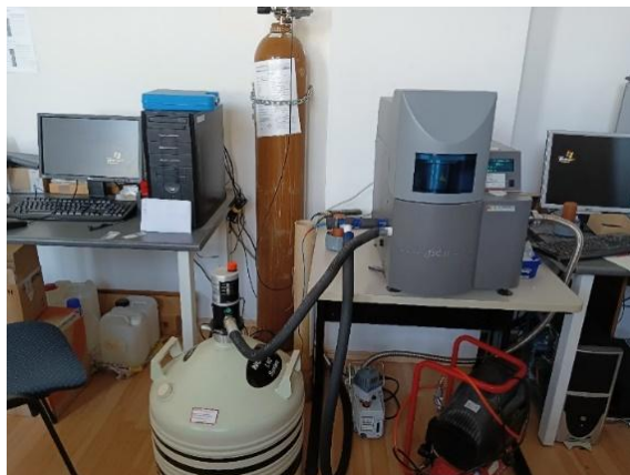
Figure 13. a) TSCII thermally stimulated depolarization instrument, b) Schematic illustration of the thermally stimulated depolarization (TSD) measurement setup [106].
