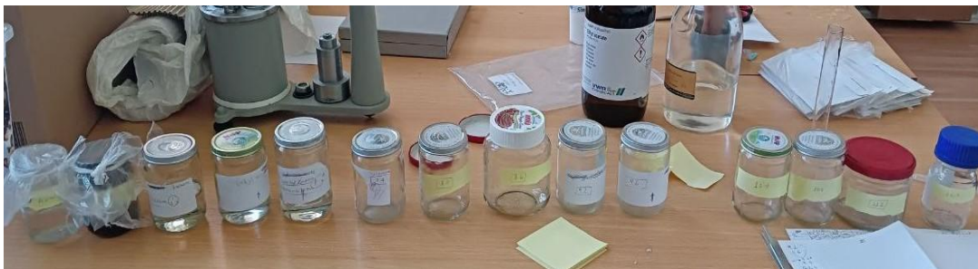
Figure 9. Swelling of polymer samples in jars of different solvents and mixture solvents.
