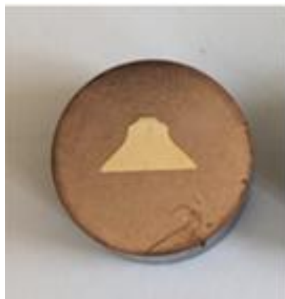
Figure 13. Sectioned MP159 probe sample after metallographic preparation (grinding and polishing), showing the exposed longitudinal cross-section prior to etching.
