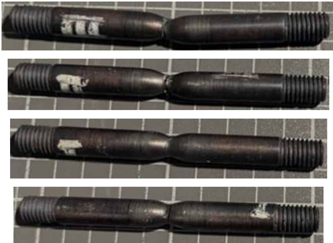
Figure 50. The mechanically simulated samples, tested at four different strain rates after failure in the Gleeble simulator: a) 2.54 s -1 , b) 25.4 s -1 , c) 254 s -1 , d) 1016 s -1 .
