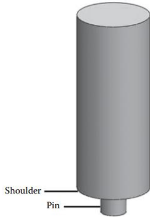
Figure 2. The FSW tool consists of a pin and a shoulder.
