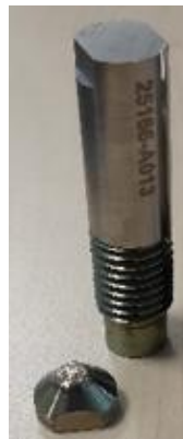
Figure 12. As-received, out-of-service MP159 SSFSW probe showing the failed tip region. The affected (failed) section was subsequently sectioned from the remainder of the probe for detailed characterisation.
